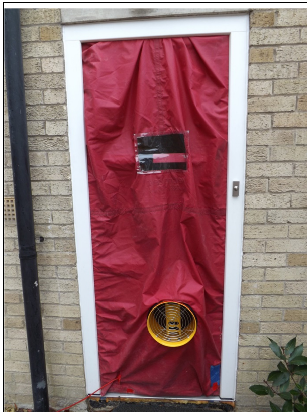
P2) External view of test equipment mounted in front entrance doorway
