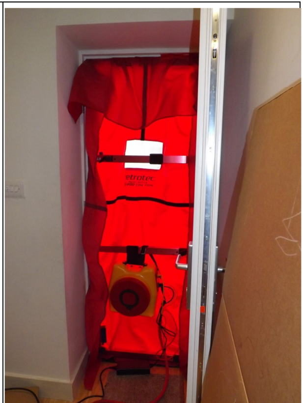
P3) Internal view of test equipment mounted in front entrance doorway
